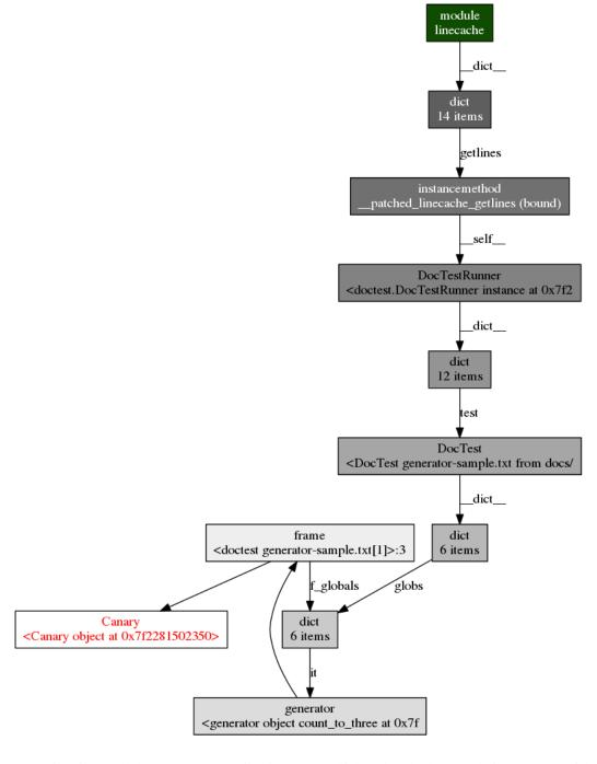
To a first approximation, modules are garbage-collection roots, which makes the latter technique most useful.
